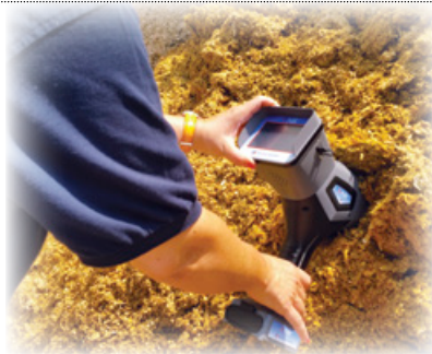
▲ Portable, instant results for: ADF, NDF, Ash, Protein, Starch, Moisture, Crude Fat and Crude Fiber.
